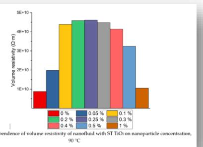
Figure 10. Dependence of volume resistivity of nanofluid with ST TiO<sub>2</sub> on nanoparticle concentration, 90 °C
